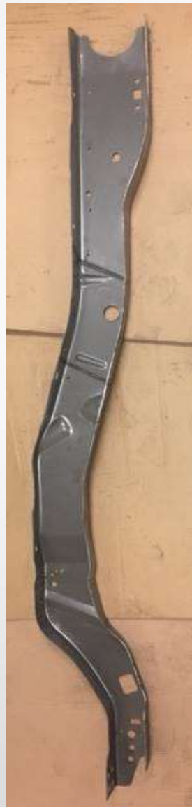
F150 Laser Welded Frame Rails
