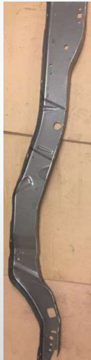
F150 Laser Welded Frame Rails
