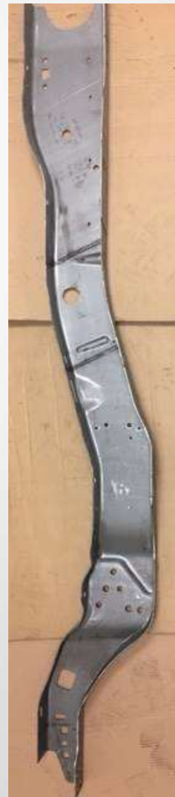
F150 Laser Welded Frame Rails
