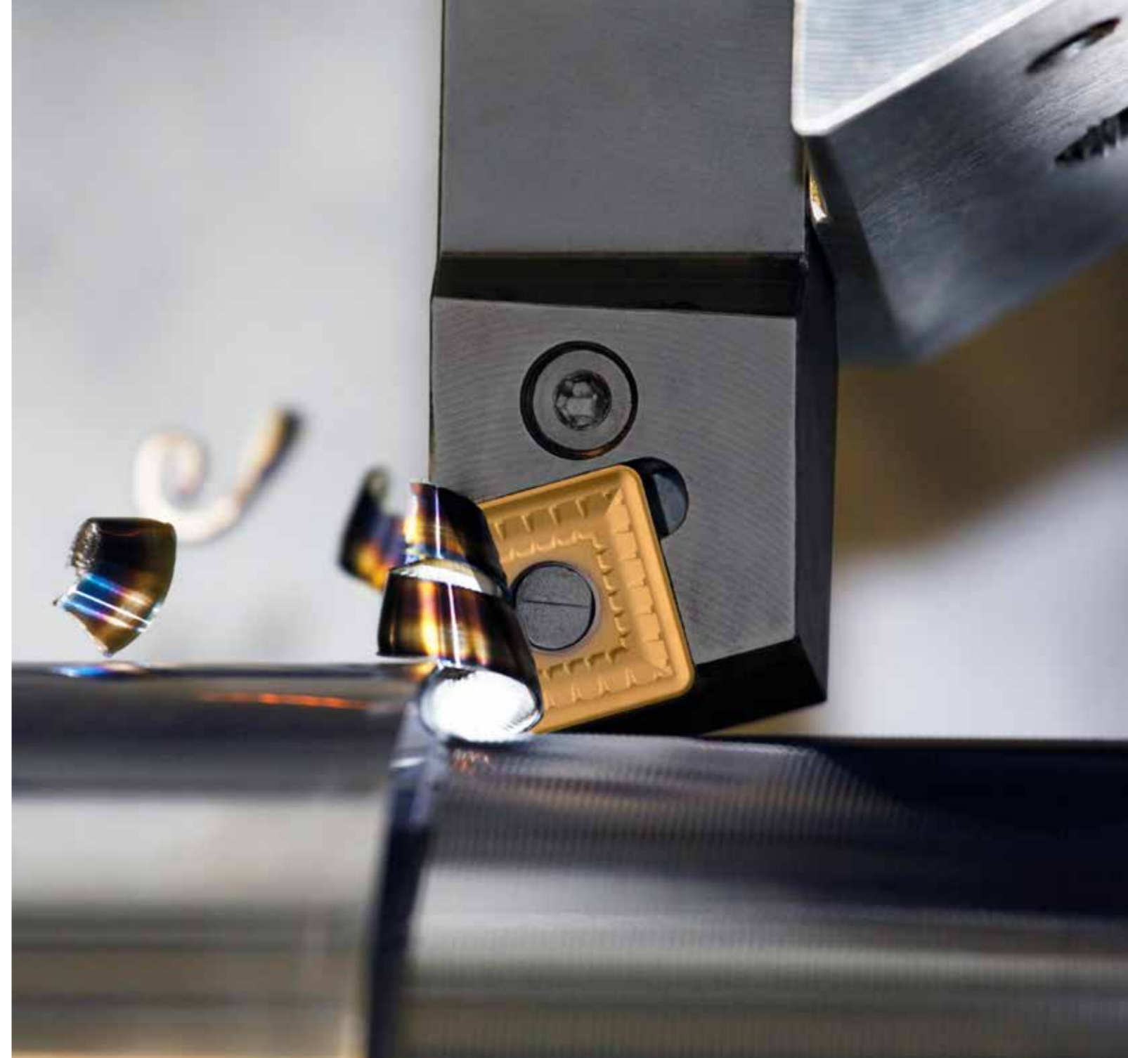
CNMG120408E- FM:T8430 FM geometry with positive design for fine-finish to semi- rough machining in steel, stainless steel and cast iron, and superalloys in continuous and slightly inter- rupted machining.
